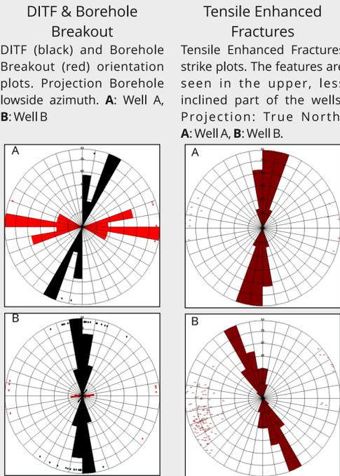
DITF (black) and Borehole Breakout (red) orientation plots. Projection Borehole lowside azimuth. A: Well A, B: Well B
