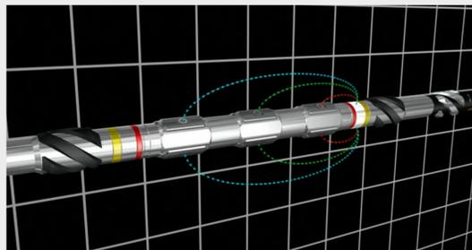
Figure 5: Sketch showing the work principle of a LWD Resistivity tool. Example of the Halliburton AFR tool. Courtesy of Halliburton Inc.
