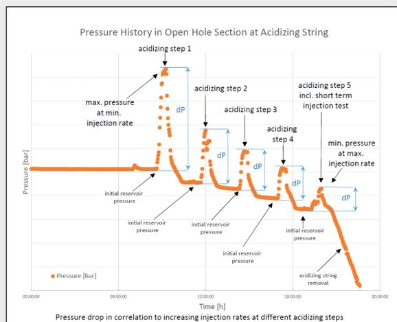
Figure 7: Injection pressure at acidizing string of acidizing fluid versus time in well A.
